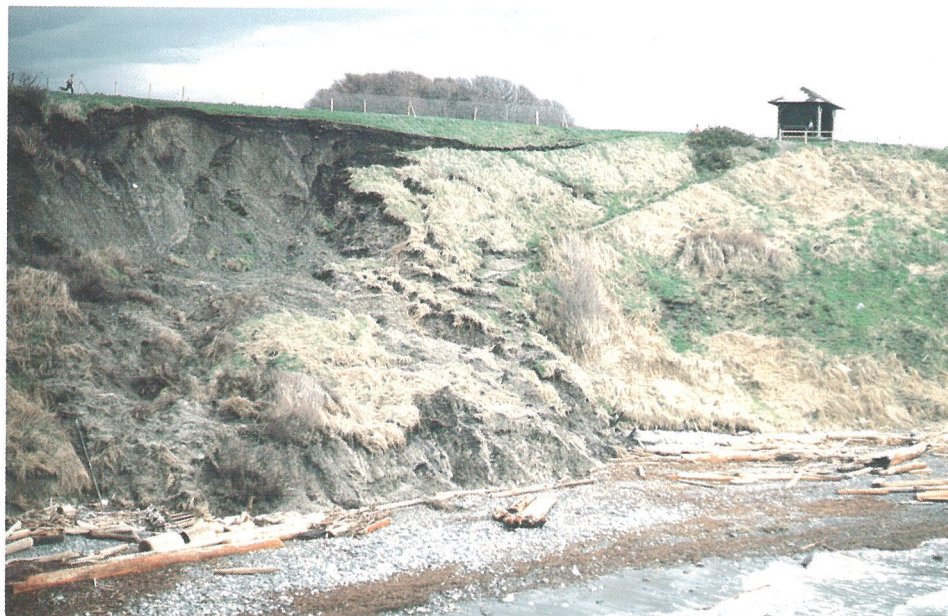
A small landslide is the result of toe erosion of a steep soil bank by wave action
