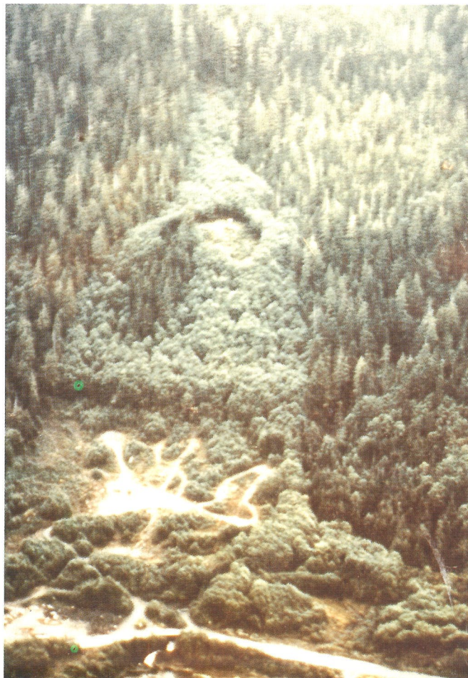
Hillslope scars and trees of the same age indicate debris slide activity
