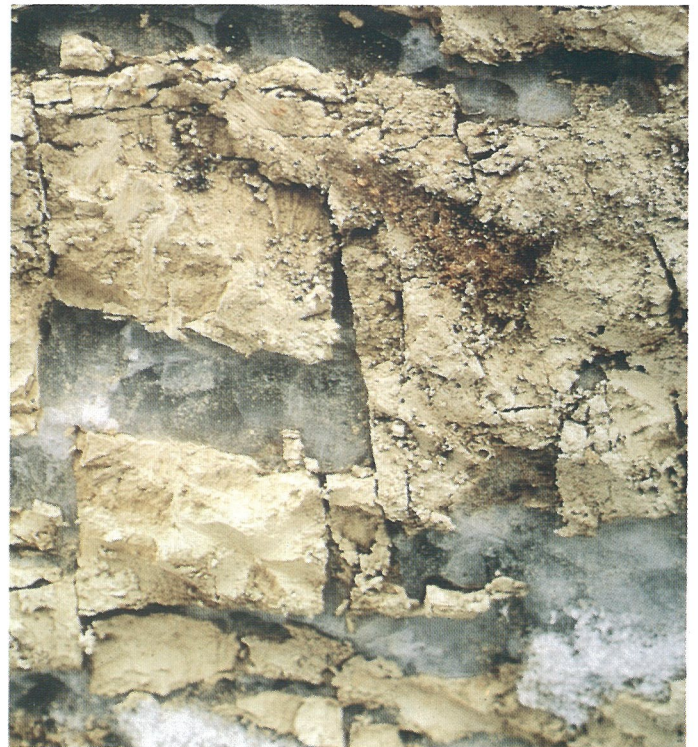
Ground ice interbedded with frozen silt
