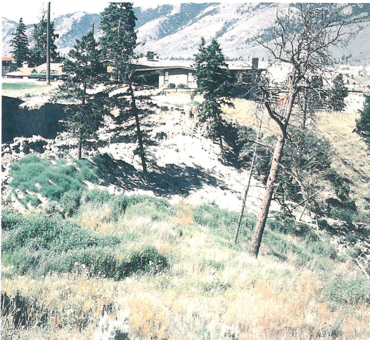
“Drunken” trees (trees leaning in all directions) indicate slope movement
