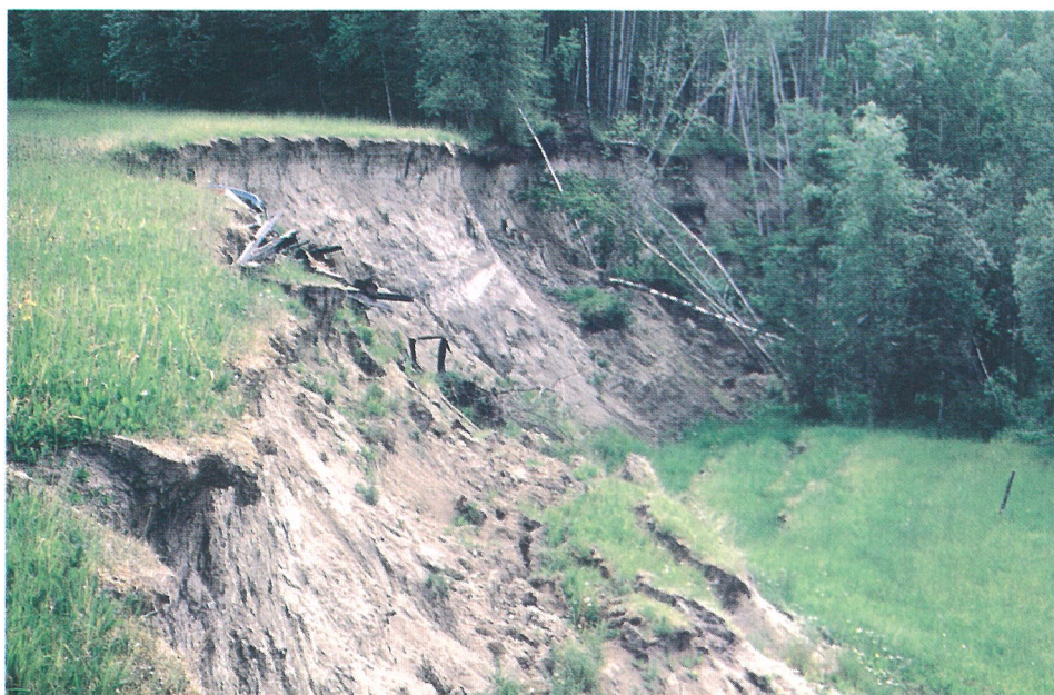
Crescent shaped scarp in fine grained soil
