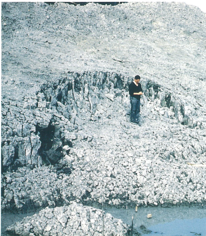
An example of a small rotational earth slump in glacial marine clay
